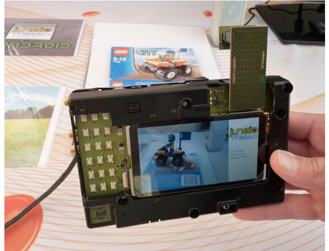
ST-Ericsson's augmented reality development board shows adaptive content fitting and flowing with the user's perspective.
