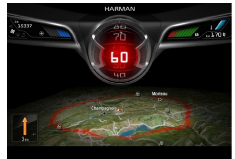
Fig. 2: Study of a main display for an e-car. The red circle marks the driving range without recharging. Source: Harman
