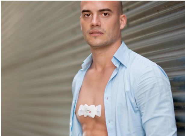
The body patch integrating an ultra-low power electrocardiogram (ECG) chip and a Bluetooth Low Energy (BLE) radio for long-term monitoring in health.
