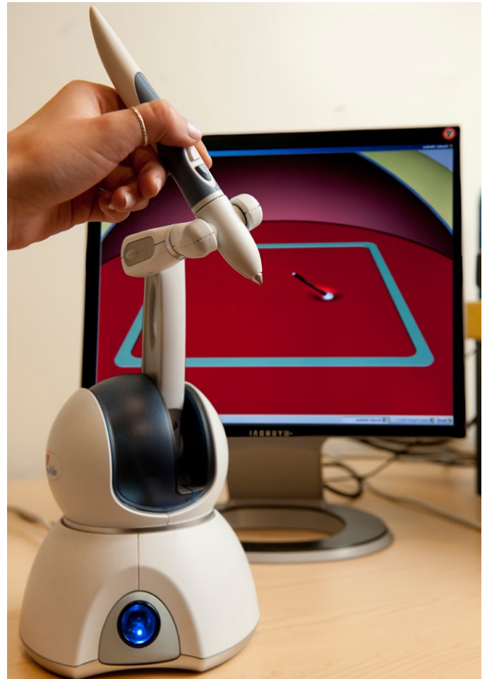
The virtual surgical haptic system.
